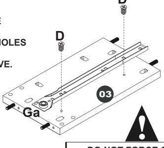
DO NOT FORCE OR OVER-TIGHTEN THE SCREWS. THIS COULD DAMAGE THE PANEL.
