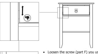
Loosen the screw (part F) you used to install the drawer runner to the side panel (parts 02 or 03), depending on the side (left or right), as shown.
