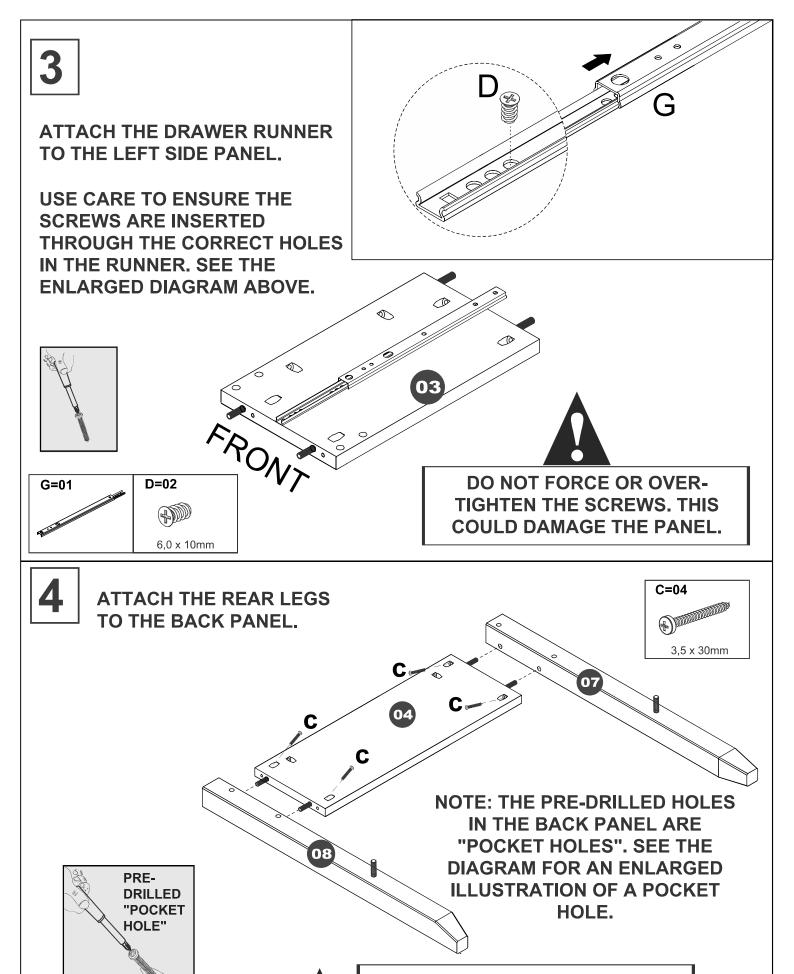
DO NOT FORCE OR OVER-TIGHTEN THE SCREWS. THIS COULD DAMAGE THE PANEL AND/OR LEGS.
