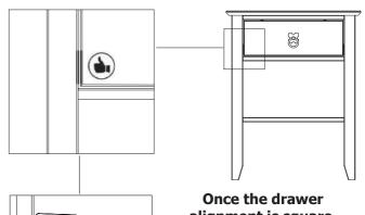
alignment is square, secure the position of the drawer runners to the side panels by re-tightening the part F screw.
