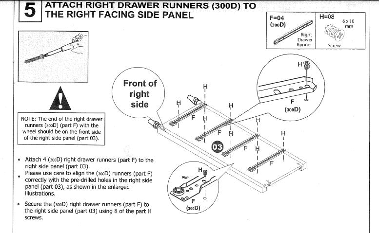
Screws (part H) should just be tight. Do not try to force or over-tighten as this may cause damage to the panel or runners.
