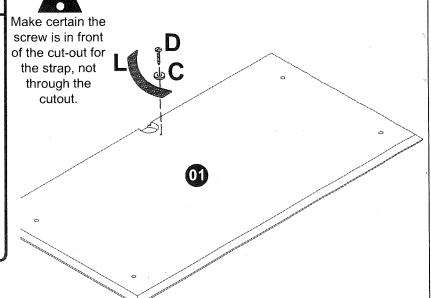
Attach the Anti-tip Safety Strap (part L) to the Top (part 01):
