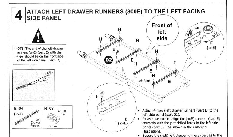
Screws (part H) should just be tight. Do not try to force or over-tighten as this may cause damage to the panel or runners.
