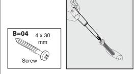
NOTE: It is easier to secure the top (part 01) with the screws (part B) with the the unit turned over (upside down) and on a hard, clean surface.
