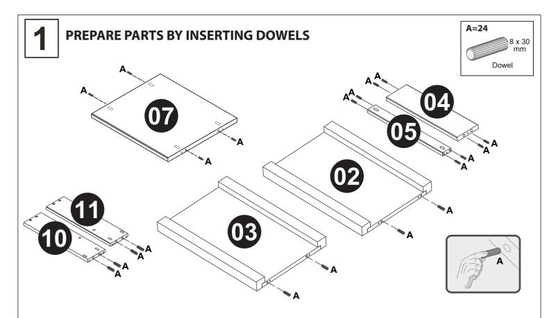
Prepare the parts for assembly by inserting dowels (part A) into the pre-drilled dowel holes in the following parts:
