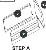
Align the Quick-2-Connect pins in the 2 drawer sides (part 7) with the pre-drilled holes in the drawer front (part 12) and push the parts together.
