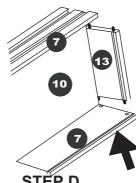
STEP D Align the Quick-2-Connect pins in the drawer back (part 13) with the pre-drilled holes in the drawer sides (part 7) <u>AND insert</u> the back of the drawer bottom (part 10) into the groove in the <u>drawer back (part 13)</u>. Then push the parts together.
