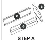
Align the Quick-2-Connect pins in the 2 drawer sides (part 6) with the pre-drilled holes in the drawer front (part 8) and push the parts together.
