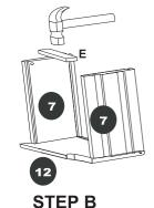
Place the wooden strike block (part E) on the end of each of the 2 drawer sides (part 7). Using a hammer or rubber mallet, tap the wooden strike
